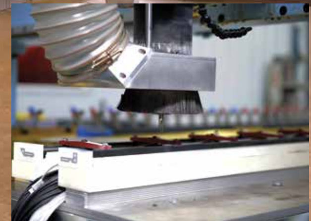
Windows and doors equipped with Thermal Evolution™ technology feature fiber-reinforced polymer (FRP) isolators. These isolators are precision machined to nest perfectly within Hope's traditional hot-rolled solid steel frame profiles where they are permanently bonded.
