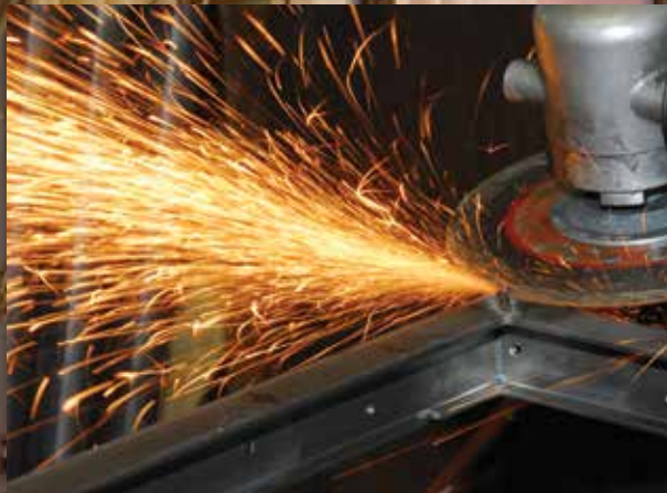
The slag that forms at welded joints is ground and sanded smooth until visually imperceptible. Windows and doors appear to have been made from a single piece of solid steel or bronze.
