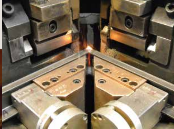
Steel profiles are joined by fusion welding, a process that fuses the steel together, forming one continuous frame.
